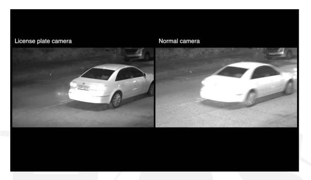
Number Plate camera recording with headlights on
